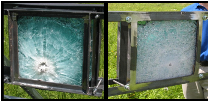
50 cal API round penetrates thick glass laminate
